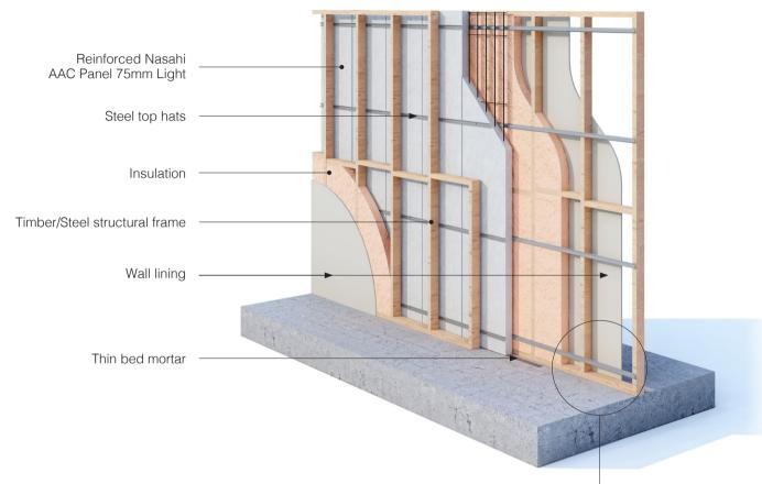
The Walsc Inter-tenancy Continuous Wall System offers a steel top hat connection where the reinforced Nasahi AAC Panel 75mm Light is secured to the structural frame with horizontal steel top hats as shown. Walsc AAC Adhesive is applied to the vertical edges where there is an adjoining panel.
